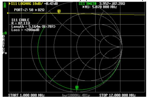
And here is big range, exist only 2 points near for calculation (marker 1 and marker 2) but bilinear interpolation calculate R = 81.74 Om very close result
