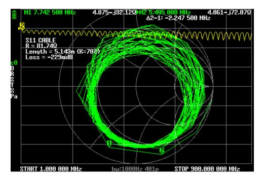
Added cable loss measure at active marker point, simple use S11 loss / 2
